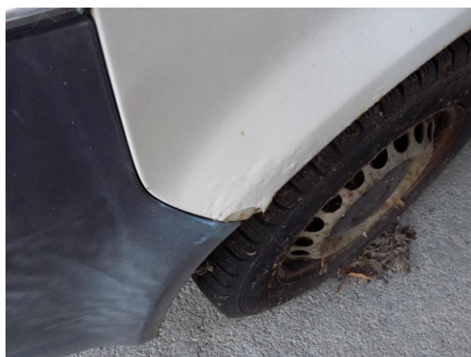
4. Volkswagen transporter – pojava korozije
